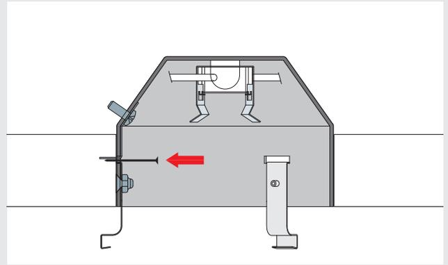
**2:** Install the transformer and then push the armature in place in the Troldtekt panel using pins.
