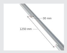
A: Make cuts as shown to enable installation in the two C60 profiles which will carry the access panel.
