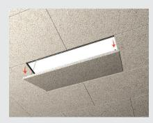
**F:** Release the snap hook to open the access panel completely.
