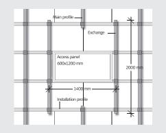
Load bearing replacement with 1 main profile interrupted
